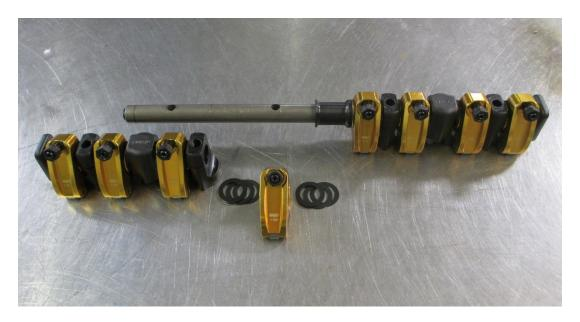
Fig. 5 - Rocker Assembly with Rocker Removed and Spacers Shown
