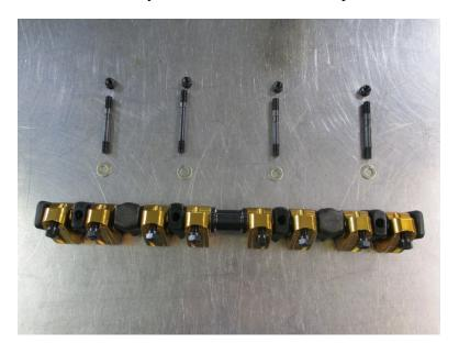
Fig. 3 - Disassembled Rocker Studs
