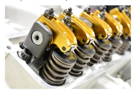
Fig. 7 - Finished Rocker Assembly
