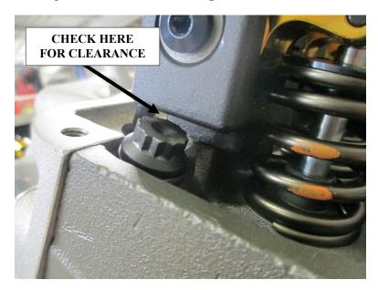
Fig. 6 - Bolt Head Clearance
